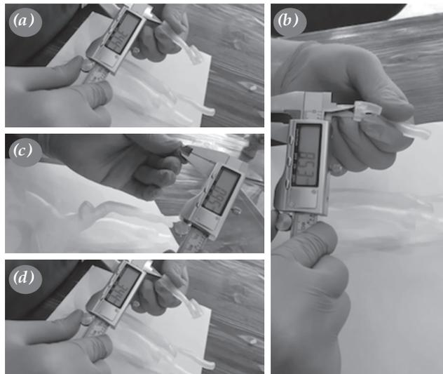
**Figure 3.** Manuel measurements of 3D printed physical models with a digital caliper. (a) Distal internal carotid artery inner diameter measured with a digital caliper. (b) Proximal internal carotid artery inner diameter measured with a digital caliper. (c) Carotid narrowing lumen diameter with a digital caliper. (d) Distal internal carotid artery inner lumen diameter measured with a digital caliper.
